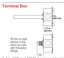
A 4 in. (100 mm) NEMA 1 octagonal terminal box is mounted on a flange or a threaded fitting. Boxes have <sup>1</sup>/<sub>2</sub> in. (13 mm) conduit knockouts for electrical connection. Hazardous location (NEMA 4 and NEMA 7) terminal boxes are also available. Contact your Watlow representative for details. Terminal boxes are available on <sup>1</sup>/<sub>2</sub> in. (13 mm) through 1 in. (25 mm) diameter FIREROD heaters. To order, specify **terminal box** and **NEMA type**.
