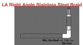
An LA right angle stainless steel braid is provided for wiring convenience. It protects leads from abrasion against sharp edges.
