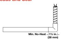
An LA right angle stainless steel hose with PTFE leads and a seal is the ultimate combination for providing abrasion protection and a moisture resistant seal with wiring convenience. Unless specified, a 12 in. (305 mm) hose is supplied. Leads are 2 in. (51 mm) longer than the hose but longer leads are available. This seal is effective to 392°F (200°C) under continuous operation.
