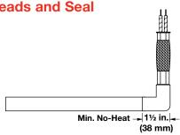
The LA right angle stainless steel braid with PTFE leads and seal is Watlow's most flexible lead protection with a moisture resistant PTFE seal and wiring convenience. Unless specified, a 12 in. (305 mm) braid is supplied. Leads are 2 in. (51 mm) longer than the braid, but longer leads are available. This seal is effective up to 392°F (200°C) under continuous operation.
