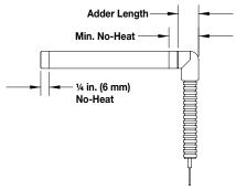
A right angle stainless steel hose is provided for wiring convenience. It protects leads from abrasion against sharp edges.
