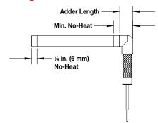
A right angle stainless steel braid is provided for wiring convenience. It protects leads from abrasion against sharp edges.
