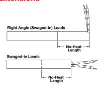
No-heat extensions are recommended in applications where leads may be exposed to excessive heat and require a cooler lead end. They are also used when heat is not required along the entire length of the FIREROD.
