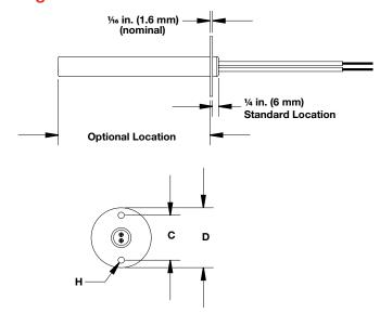
Stainless steel flanges are a convenient mounting method and can be used to position a heater within an application. The standard location is <sup>1</sup>/<sub>4</sub> in. (6 mm) from the lead end. However, a specific location may be requested in any location along the no-heat section. Unless specified, flanges are staked to the sheath.
