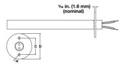
Stainless steel flanges are a convenient mounting method to position a heater within an application. The flange is staked on and located  $^{1}/_{4}$  in. (6 mm) from the lead end. The flange can be located up to  $2^{1}/_{4}$  in. (57 mm) from the lead end if it is over a no-heat section. Use this option in combination with most LA configurations.
