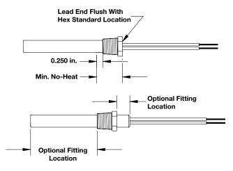
Threaded fittings allow fast, water-tight heater installation into a threaded hole. Standard fittings are 304 stainless steel and welded to the heater sheath. Other materials are available upon request. Double threaded fittings are also available.
