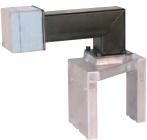
**"L" Shaped Bronze, Brass or Aluminum Cast-In Heaters** are sold as individual units. They are normally supplied with a moisture resistant junction box. Also available with explosion resistant or cast-on junction box, fitted with convoluted wire braided hose and high temperature lead wire. If required, specify. For additional terminations, see pages 3-54 and 3-55.
