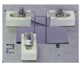
flag type terminal. This design makes use of the flag type terminal exiting the heater that is then bent over a ceramic mounting block with a vertically mounted stud. This approach uses the stud as a means of easy connection, but not as a current carrying device. Therefore, higher
