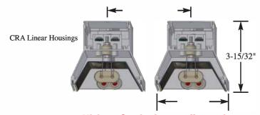
Minimum Spacing between Heaters in Array Assemblies ("D" Dim.) and CRA Linear Housings
