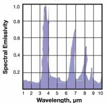
**WAVELENGTH CONTROL** – The very low heat transmission losses through the clear quartz material of the twin bore heaters allow Tempco's engineers to carefully design the peak emitted wavelength of these heaters to match the peak absorption wavelength for a given material or application. By modifying the temperature of the E-mitter, its peak emitted wavelength will change according to Wien's displacement law (see page 7-101). All E-
