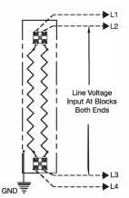
**Double End Heater Wiring Dual Element Parallel Wired**
