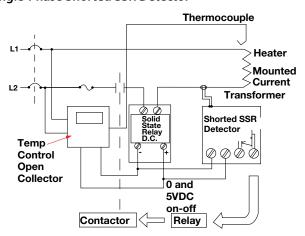
**Note:** Semiconductor power switching devices are not legal for over temperature limit or safety devices. For limit and safety devices you must have a positive mechanical break of all electrically hot legs simultaneously.
