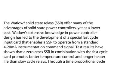
Both low and high voltage models are available from 24 up to 530VAC. All ac output models include back to back Silicon Controlled Rectifiers (SCRs) for a more rugged design than the traditional triac based SSR. The internal design allows it to handle high currents and the harsh electrical environments of heavy industry. Watlow also offers a switched VDC model for dc heating applications.
