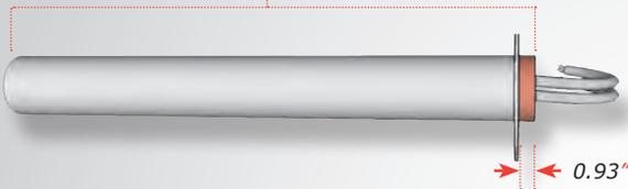
Heater size at **Maximum** Length tolerance.
