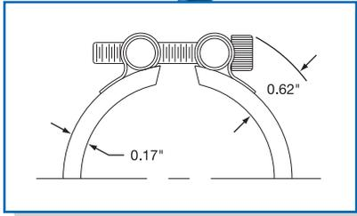
High operating temperatures require superior clamping force to maintain ultimate contact between the inside diameter of the band heater and the barrel, which is essential for maximum heater operating life. Only Tempco's Mi-Plus offers you this unique Built-In Strap feature.
