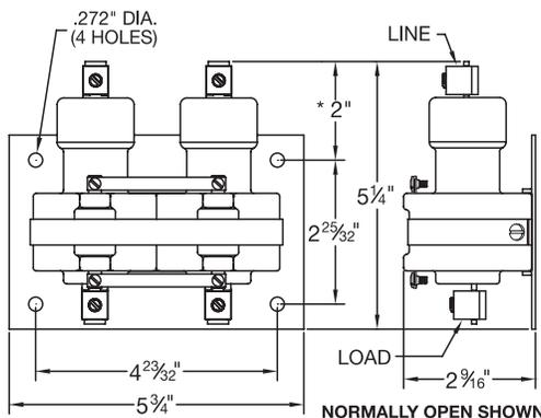
\* THIS DIMENSION IS 1 5/16" FOR NORMALLY CLOSED TWO POLE UNITS
