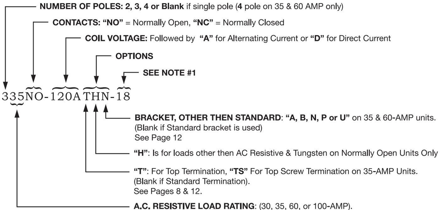
NOTES: 1) Other designations are -1 thru -99. These are suffix numbers, and are reserved for units with dead special detail, construction and/or features. -11 MOV on coil (see page 20), -13 MOV & metal strap, -17 DIN rail mount, -20 DIN rail & metal strap (see page 12), -18 metal strap (see page 9). (See example #2).
