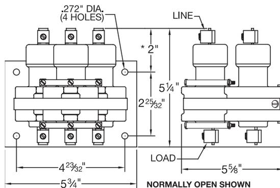
\* THIS DIMENSION IS 1 5/16" FOR NORMALLY CLOSED THREE POLE UNITS
