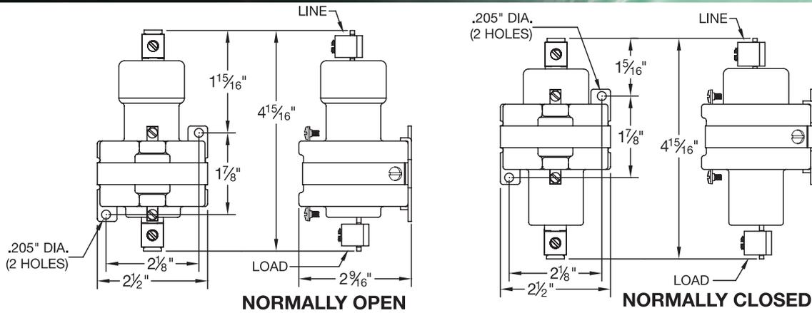
For UV Curing, and Various High Voltage applications. Available in Single Pole, Normally Open, and Normally Closed Units. The coils utilize 6-32 Wire Binding Screws, and the Contacts use Compression type terminals for #2 thru #8 AWG wire.
